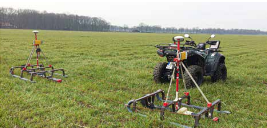
EMI measurement setup as used in POTENTIAL: the quad simultaneously pulls 2 sleds containing one EMI device and GPS antenna each. Design of the sleds: Forschungszentrum Jülich GmbH.
