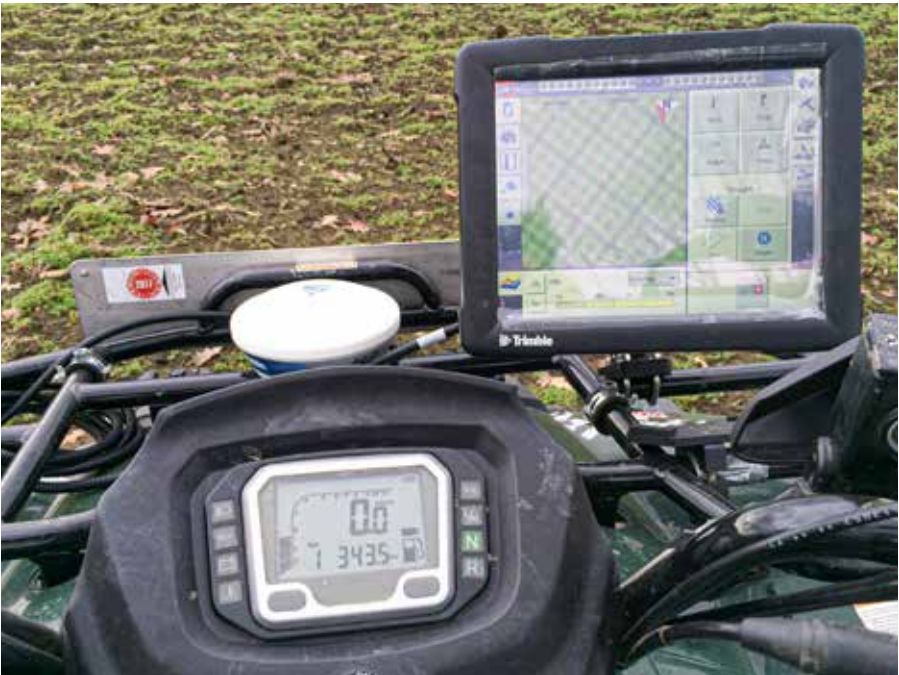
The quad driver uses the high-precision GPS equipment to plan and follow his/her measurement track.
