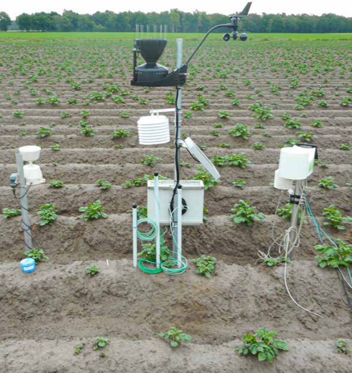
Weather station and different soil sensors as installed on the field of Jacob Van Den Borne in the Netherlands in 2019 (Field nr 12)
