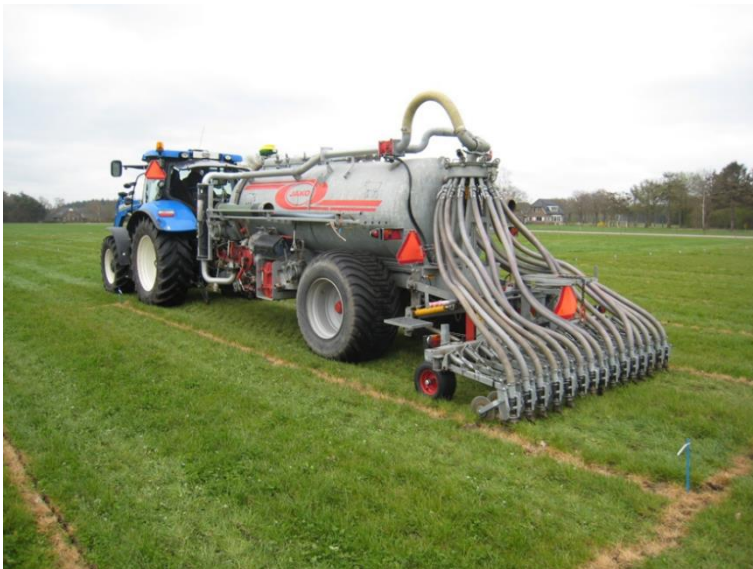
Photo 4 Injector of WUR Unifarm which was designed for the application of animal slurries. It was adjusted for application of cattle slurry on grassland with slots distanced at 25 cm in this photograph.
