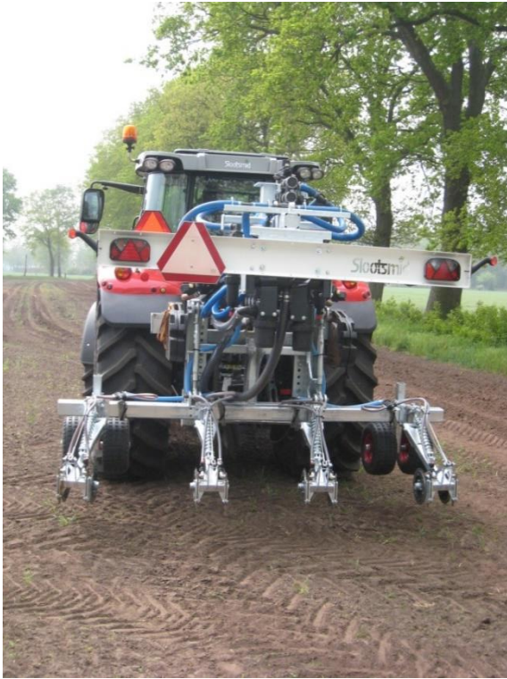
Photo 3 Injector designed for biobased fertilising products. Injector was built by Slootsmid 28 in 2020 and is designed for specific use in field experiments and/or fertilisation of small plots. The design was aimed at mitigating/minimising ammonia losses.
