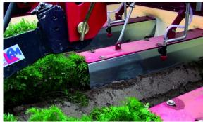
Figure 7A Sprayer for row specific application F
