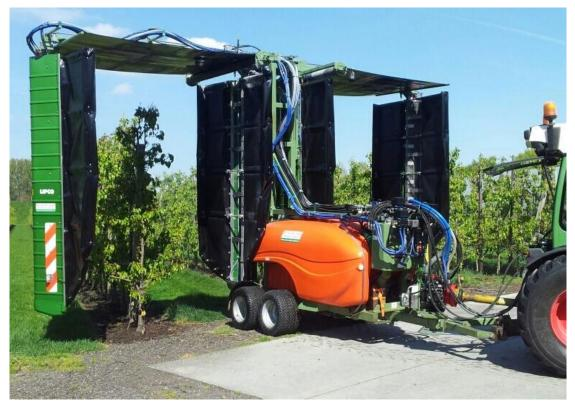
Figure 9 Two row tunnel-sprayer with recirculation-system
