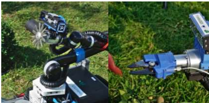
Figure 2: TrimBot2020 topiary trimming tool and rose clipping tool (source: www.wur.nl )
