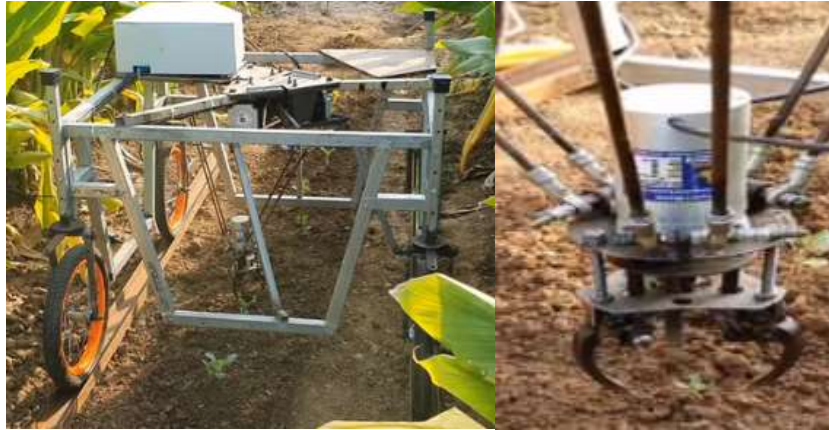
Figure 4: The Nindamani robot and his gripper (source: www.hackster.io )
