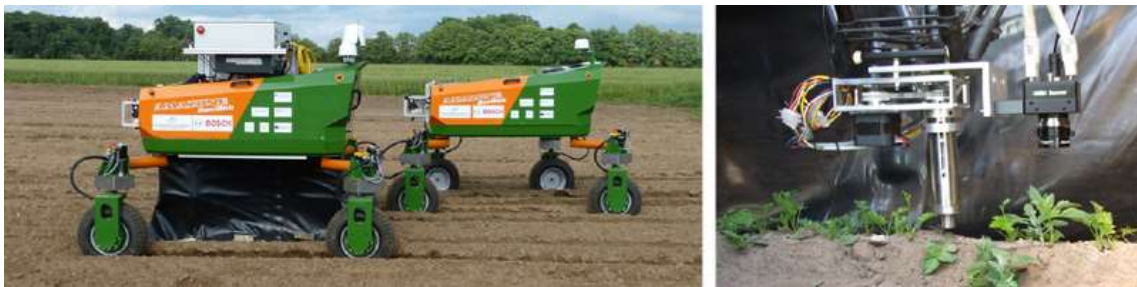
Figure 3: BoniRob robot (Amazone and Bosch) and his tube stamp (source: www.researchgate.net )
